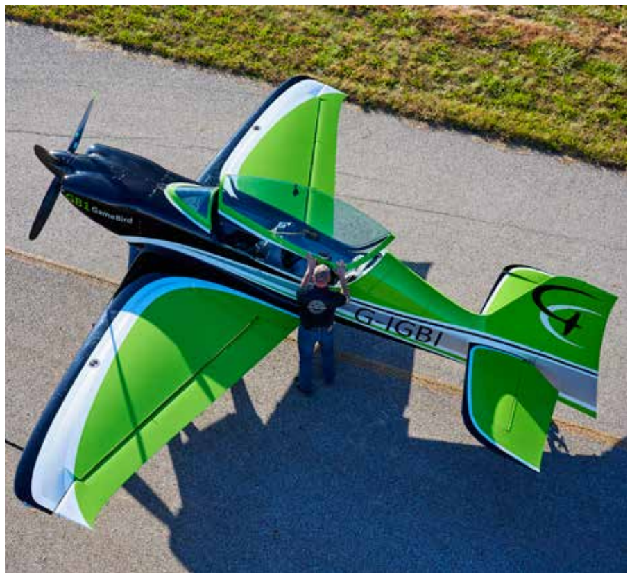
COMPOSITE CONSTRUCTION allows curved contours from the wing tips (above left and right) to the rakish tail. The prototype (below) was first registered in England and still carries a British G registration.
