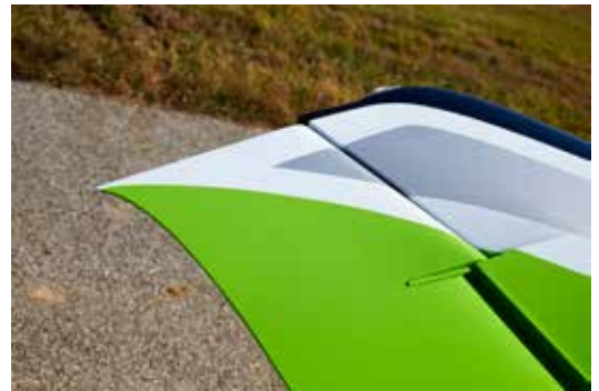
COMPOSITE CONSTRUCTION allows curved contours from the wing tips (above left and right) to the rakish tail. The prototype (below) was first registered in England and still carries a British G registration.
